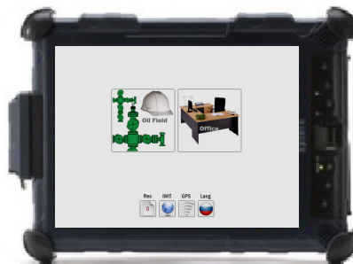
Figure 4 – iWITNotePad touch screen handheld tablet PC for entry of data from the wellsite directly into iWIT.
